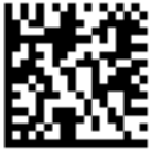
Figure 2.1. Example Data Matrix Symbol
